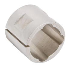
SureMotion bore reducer, clamping, stainless steel body, 7/8in outside diameter, 11/16in inside diameter.
