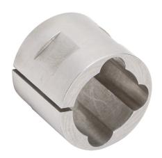
SureMotion bore reducer, clamping, stainless steel body, 7/8in outside diameter, 5/8in inside diameter.
