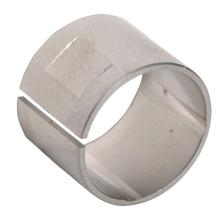
SureMotion bore reducer, clamping, stainless steel body, 5/8in outside diameter, 9/16in inside diameter.
