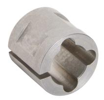
SureMotion bore reducer, clamping, stainless steel body, 1/2in outside diameter, 5/16in inside diameter.
