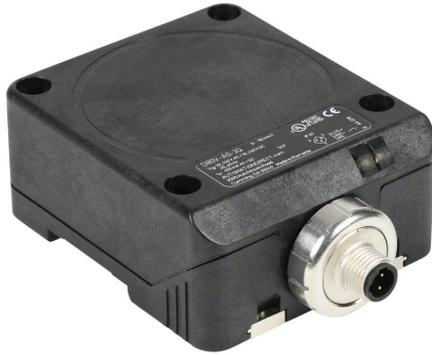
ProSense inductive proximity sensor, rectangular, 80 x 40 x 92mm body, polyphenylene ether housing, N.O. output, 50mm sensing distance, flush, 25 Hz switching frequency, IP67, 3-pin 1/2in - 20UNF thread.
