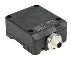
ProSense inductive proximity sensor, rectangular,  $80 \times 40 \times 92$ mm body, polyphenylene ether housing, N.O. output, 50mm sensing distance, flush, 25 Hz switching frequency, IP67, 3-pin 1/2in - 20UNF thread.
