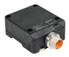
ProSense inductive proximity sensor, rectangular,  $80 \times 40 \times 92$ mm body, polyphenylene ether housing, N.O. output, 50mm sensing distance, flush, 25 Hz switching frequency, IP67, 3-pin mini and 7/8in - 16UNF thread.
