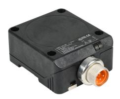
ProSense inductive proximity sensor, rectangular, 80 x 40 x 92mm body, polyphenylene ether housing, N.O. output, 50mm sensing distance, flush, 25 Hz switching frequency, IP67, 3-pin mini and 7/8in - 16UNF thread.
