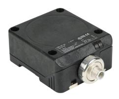
ProSense inductive proximity sensor, rectangular, 80 x 40 x 92mm body, polyphenylene ether housing, PNP, N.O. output, 50mm sensing distance, flush, 70 Hz switching frequency, IP67, 4-pin M12 quick-disconnect.
