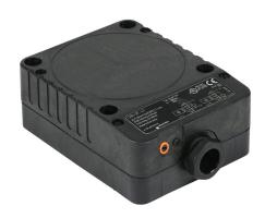
ProSense inductive proximity sensor, rectangular, 80 x 40 x 105mm body, polyphenylene ether housing, PNP, N.O./N.C. selectable output, 20-60mm sensing distance, non-flush, 100 Hz switching frequency, IP65, terminal chamber.
