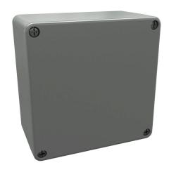
Stahlin DuraBoxx series enclosure, NEMA 1/3/3S/4X/6/6P/12,  $160 \times 160 \times 91$ mmmm (HxWxD), fiberglass reinforced polyester, Pantone 428 C glacier gray, screw cover.
