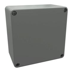
Stahlin DuraBoxx series enclosure, NEMA 1/3/3S/4X/6/6P/12, 160 x 160 x 91mmmm (HxWxD), fiberglass reinforced polyester, Pantone 428 C glacier gray, screw cover.
