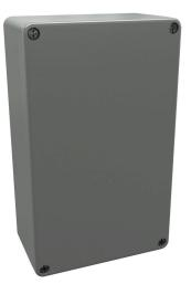
Stahlin DuraBoxx series enclosure, NEMA 1/3/3S/4X/6/6P/12, 160 x 260 x 91mm (HxWxD), fiberglass reinforced polyester, Pantone 428 C glacier gray, screw cover.
