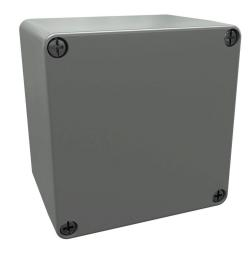
Stahlin DuraBoxx series enclosure, NEMA 1/3/3S/4X/6/6P/12, 122 x 120 x 91mm (HxWxD), fiberglass reinforced polyester, Pantone 428 C glacier gray, screw cover.
