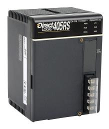
DirectLOGIC DL405 slave, (1) 5-pin terminal block port(s), serial remote I/O, external 110-220 VAC required. 24 VDC 400 mA auxiliary device power supply included.
