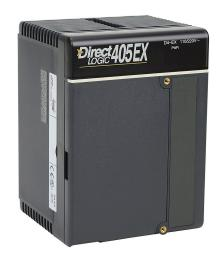
DirectLOGIC DL405 expansion unit, (1) terminal strip port(s), local expansion I/O, external 110-220 VAC required. 24 VDC 400mA auxiliary device power supply included. Requires D4-EXCBL-1 or D4-EXCBL-2 external I/O expansion cable.
