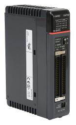
DirectLOGIC DL405 discrete output module, 64-point, 5-24 VDC, sinking, 8 common(s), 8 point(s) per common, 0.1A/point, 1A/ common, 8A/module. Requires ZIPLink pre-wired cable.
