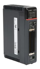
DirectLOGIC DL405 discrete output module, 64-point, 5-24 VDC, sinking, 8 common(s), 8 point(s) per common, 0.1A/point, 1A/common, 8A/module. Requires ZIPLink pre-wired cable.
