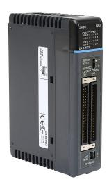
DirectLOGIC DL405 discrete input module, 64-point, 24 VDC, sourcing, 8 isolated common(s), 8 point(s) per common.
