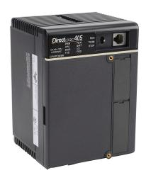
DirectLOGIC DL405 CPU, 31.5k words ladder memory, (1) RS-232 (DB15), (1) RS-232 (RJ12) and (2) RS-232/RS-422 (DB25) port(s), external 120-240 VAC required, battery included.
