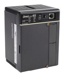
DirectLOGIC DL405 CPU, 31.5k words ladder memory, (1) RS-232 (DB15), (1) RS-232 (RJ12) and (2) RS-232/RS-422 (DB25) port(s), external 12-24 VDC required, battery included.
