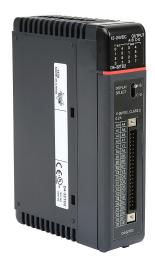
DirectLOGIC DL405 discrete output module, 32-point, 12-24 VDC, sourcing, 4 isolated common(s), 8 point(s) per common, 0.2A/point, 1A/common, 4A/module. Requires ZIPLink pre-wired cable.
