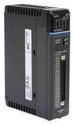
DirectLOGIC DL405 discrete input module, 32-point, 24 VDC, sinking/sourcing, 4 isolated common(s), 8 point(s) per common.
