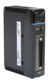
DirectLOGIC DL405 discrete input module, 32-point, 24 VDC, sinking/sourcing, 4 isolated common(s), 8 point(s) per common.
