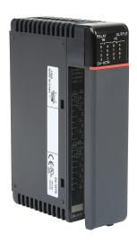
DirectLOGIC DL405 relay output module, 16-point, 6-24 VDC/6-240 VAC, (16) Form A, 2 isolated common(s), 8 point(s) per common, 1A/point, 5A/common. Removable terminal block included.
