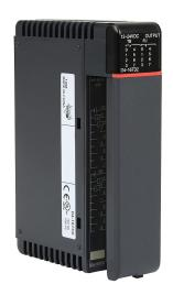
DirectLOGIC DL405 discrete output module, 16-point, 12-24 VDC, sourcing, 2 isolated common(s), 8 point(s) per common, 0.5A/point, 3A/common. Removable terminal block included.
