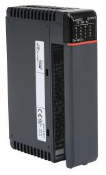
DirectLOGIC DL405 discrete output module, 16-point, 5-24 VDC, sinking, 2 common(s), 8 point(s) per common, 0.5A/point, 3A/ common. Removable terminal block included.
