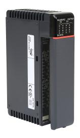
DirectLOGIC DL405 discrete output module, 16-point, 24-240 VAC, 2 isolated common(s), 8 point(s) per common, 0.5A/point, 3A/common. Removable terminal block included.
