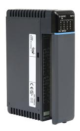
DirectLOGIC DL405 discrete input module, 16-point, 12-24 VDC, sourcing, 2 isolated common(s), 8 point(s) per common. Removable terminal block included.
