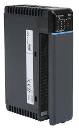
DirectLOGIC DL405 discrete input module, 16-point, 12-24 VDC, sourcing, fast response, 2 isolated common(s), 8 point(s) per common. Removable terminal block included.
