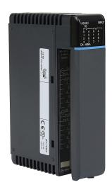
DirectLOGIC DL405 discrete input module, 16-point, 120 VAC, 2 isolated common(s), 8 point(s) per common. Removable terminal block included.
