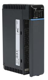
DirectLOGIC DL405 discrete input module, 16-point, 120 VAC, 2 isolated common(s), 8 point(s) per common. Removable terminal block included.
