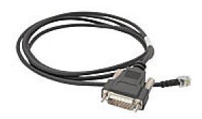
AutomationDirect communication cable, 6-pin RJ12 to 15-pin male D-sub, shielded, 2m/6.6ft cable length. For use with DV-1000 or C-more Micro panels and any DL405 CPU.
