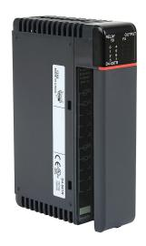
DirectLOGIC DL405 relay output module, 8-point, 6-24 VDC/6-240 VAC, (8) Form A, 2 isolated common(s), 4 point(s) per common, 2A/point, 5A/common. Removable terminal block included.
