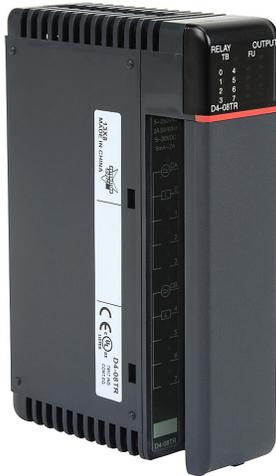
DirectLOGIC DL405 relay output module, 8-point, 6-24 VDC/6-240 VAC, (8) Form A, 2 isolated common(s), 4 point(s) per common, 2A/point, 5A/common. Removable terminal block included.
