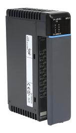
DL405 discrete input module, 8-point, 24-48 VDC, sinking/sourcing, 8 isolated common(s), 1 point(s) per common. Removable terminal block included.
