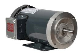
Marathon XRI premium efficiency AC induction motor, general purpose, inverter rated and 4-in-1, 2hp, 3-phase, 230/460 VAC, suitable for 208 VAC at 60 Hz, 3600rpm, TEFC, NEMA 56HC frame, rolled steel, C-face/removable rigid base mount.
