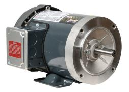
Marathon XRI premium efficiency AC induction motor, general purpose, inverter rated and 4-in-1, 1hp, 3-phase, 230/460 VAC, suitable for 208 VAC at 60 Hz, 3600rpm, TEFC, NEMA 56C frame, rolled steel, C-face/removable rigid base mount.
