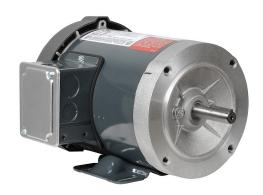
Marathon XRI standard efficiency AC induction motor, general purpose, inverter rated and 4-in-1, 3/4hp, 3-phase, 208-230/460 VAC, 3600rpm, TEFC, 56C frame, rolled steel, C-face/removable rigid base mount.
