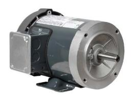
Marathon XRI standard efficiency AC induction motor, general purpose, inverter rated and 4-in-1, 1/2hp, 3-phase, 208-230/460 VAC, 3600rpm, TEFC, 56C frame, rolled steel, C-face/removable rigid base mount.
