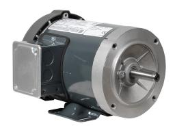
Marathon XRI standard efficiency AC induction motor, general purpose, inverter rated and 4-in-1, 1/2hp, 3-phase, 208-230/460 VAC, 3600rpm, TEFC, NEMA 56C frame, rolled steel, C-face/removable rigid base mount.
