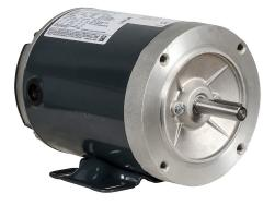
Marathon XRI standard efficiency AC induction motor, general purpose, 4-in-1 and high-performance inverter duty, 1/3hp, 3-phase, 208-230/460 VAC, 3600rpm, TENV, NEMA 56C frame, rolled steel, C-face/removable rigid base mount.
