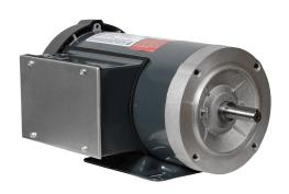
Marathon standard efficiency AC induction motor, general purpose and 4-in-1, 3hp, 1-phase, 208-230 VAC, 3600rpm, TEFC, NEMA 56HC frame, rolled steel, C-face/removable rigid base mount.
