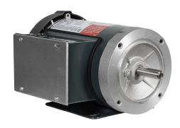
Marathon standard efficiency AC induction motor, general purpose and 4-in-1, 2hp, 1-phase, 115/208-230 VAC, 3600rpm, TEFC, 56HC frame, rolled steel, C-face/removable rigid base mount.
