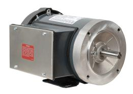
Marathon standard efficiency AC induction motor, general purpose and 4-in-1, 1-1/2hp, 1-phase, 115/208-230 VAC, 3600rpm, TEFC, 56C frame, rolled steel, C-face/removable rigid base mount.
