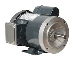
Marathon standard efficiency AC induction motor, general purpose and 4-in-1, 3/4hp, 1-phase, 115/208-230 VAC, 3600rpm, TEFC, 56C frame, rolled steel, C-face/removable rigid base mount.
