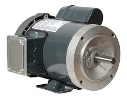
Marathon standard efficiency AC induction motor, general purpose and 4-in-1, 3/4hp, 1-phase, 115/208-230 VAC, 3600rpm, TEFC, NEMA 56C frame, rolled steel, C-face/removable rigid base mount.
