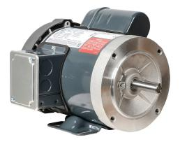
Marathon standard efficiency AC induction motor, general purpose and 4-in-1, 1/2hp, 1-phase, 115/208-230 VAC, 3600rpm, TEFC, NEMA 56C frame, rolled steel, C-face/removable rigid base mount.
