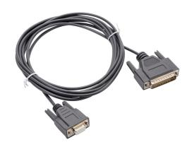
DirectLOGIC DL305 programming cable, 12ft cable length, shielded, 9-pin female D-sub to 25-pin male D-sub. For use with DL305 and DL405 CPUs and D2-DCM, D3-DCM and D4-DCM modules. D3-232-DCU module required for use with D3-330 and D3-340 CPUs.
