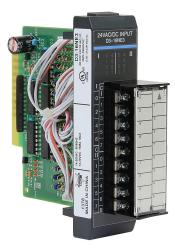
DirectLOGIC DL305 discrete input module, 16-point, 24 VAC/VDC, sinking/sourcing, 2 isolated common(s), 8 point(s) per common. Removable terminal block included.
