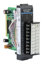
DirectLOGIC DL305 discrete input module, 16-point, 24 VDC, sourcing, 2 common(s), 4 point(s) per common. Removable terminal block included.
