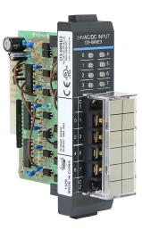
DL305 discrete input module, 8-point, 24 VAC/VDC, sinking/ sourcing, 2 isolated common(s), 4 point(s) per common. Nonremovable terminal block included.
