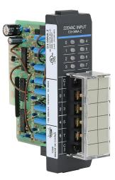
DirectLOGIC DL305 discrete input module, 8-point, 240 VAC, 2 isolated common(s), 4 point(s) per common. Non-removable terminal block included.
