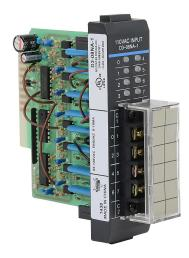
DirectLOGIC DL305 discrete input module, 8-point, 120 VAC, 2 isolated common(s), 4 point(s) per common. Non-removable terminal block included.
