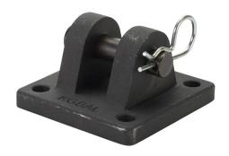
NITRA cylinder rear clevis bracket, steel. For use with 2.5in bore D2 series NFPA cylinders. Mounting hardware included.
