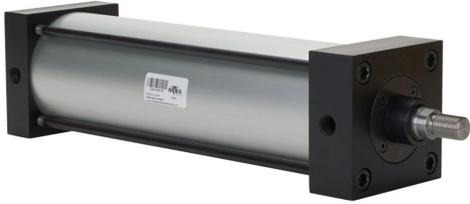
NITRA pneumatic cylinder, NFPA tie rod, 4in bore, 1in rod diameter, 12in stroke, double acting, magnetic piston, tapped end caps mount.
