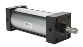
NITRA pneumatic cylinder, NFPA tie rod, 4in bore, 1in rod diameter, 8in stroke, double acting, magnetic piston, front and rear adjustable cushions, tapped end caps mount.
