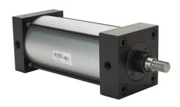
NITRA pneumatic cylinder, NFPA tie rod, 4in bore, 1in rod diameter, 7in stroke, double acting, magnetic piston, tapped end caps mount.
