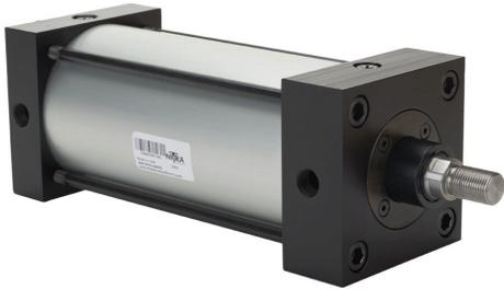
NITRA pneumatic cylinder, NFPA tie rod, 4in bore, 1in rod diameter, 7in stroke, double acting, magnetic piston, front and rear adjustable cushions, tapped end caps mount.
